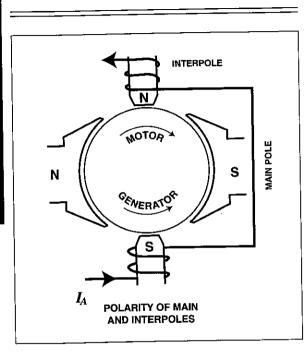
The diagram above shows the polarity of interpoles with respect to the polarity of the main poles.
